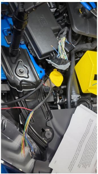
6. Identify the SSF, SSC, and SSB solenoid wires so that the 10RStager can be inserted into this interface.
